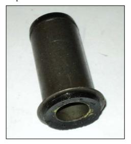
The part number is K-3026 and should be readily available as they are used on Ramblers from 1962 onwards. These aren't used on any other car, like pitman arms and idler arms – AMC-Rambler only!
