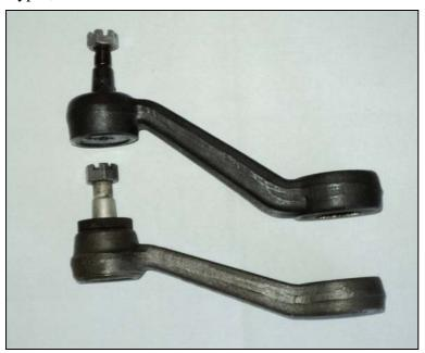
The top pitman arm is a small taper small spline arm for a Hornet
