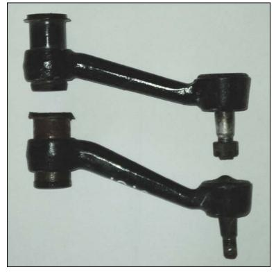
Check out the pressed in distance on these two. The top one is a power steering one off a Matador (large taper)
